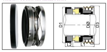
Elastomer diaphragm seals with sinusoidal wave-springs. 50mm size is routinely used as upper seal in certain "AFP" range submersible pumps, with 45mm Type 195 as the lower seal. The 65mm Type 1577 is a lower seal, and is normally paired with the 55mm Type 195. For identification purposes, please cross-reference the O.E.M. part number shown below, or enquire.
