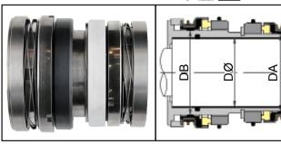
Elastomer diaphragm seals with sinusoidal wave-springs, supplied as upper and lower seals, ready mounted on a shaft sleeve, for installation directly into the bell-chamber style housing of A.B.S.\* / Pumpex\* "K" series pumps. For 25mm, 32mm or 35mm shaft sizes, please enquire.
