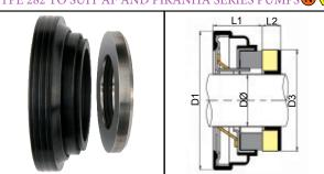
Rubber-encased upper seals primarily for "Piranha-M or -S" range submersible pumps. The lower seal is normally 25mm or 30mm Type 195 seal, detailed above. For identification purposes, please crossreference the O.E.M. part number, or enquire.
