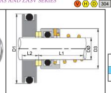
O'-Ring mounted conical spring seals with distinctive stationaries, to suit the seal chambers of "BAS, SPF, ZAS and ZASV" series spindle or screw pumps, commonly found in ship's engine rooms on oil and fuel duties. Clockwise rotation springs are standard.
