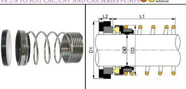
Elastomer diaphragm seals to 2.3/8" shaft size, with extended taper coil, to suit internal dimensions of Eureka® "CAC, CAV and CAX" series centrifugal pumps, widely used in marine applications.
