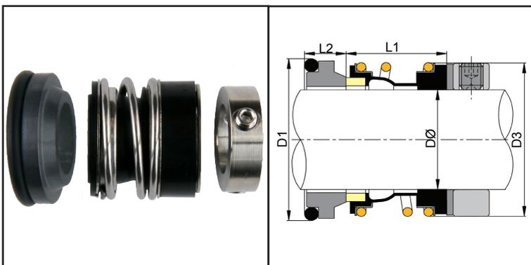
Vulcan manufacture and stock 16mm elastomer bellows seals with spacer and clamp ring to suit the Grundfos® “CP” series pumps. Widely utilised in building service applications.
