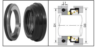
VULCAN<sup>®</sup> TYPE 28 TO SUIT HAIGH<sup>®</sup> MACERATORS **N F 304** Vulcan manufacture and stock 1.1/4" rotaries, and 1.3/4" complete seals, to suit Haigh® macerators. Rotaries have Carbon faces with Nitrile elastomers, complete seals have a Ni-Resist cast iron stationary with a Nitrile 'O'-Ring.
