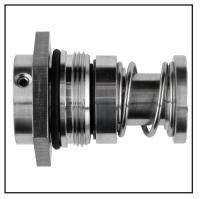
Vulcan manufacture and stock 12mm and 16mm Type 953 screw-fit semi-cartridge seals and 22mm Type 954 push-fit semi-cartridge seals to replace Grundfos\* "H-" code seals installed in CR, CRI, CRIE series vertical multi-stage pumps. Type 953 and 954 are intended for all standard clockwise rotation pumps. 16mm Type 953 is also available in "953L" format specifically for "CR15SF" models with anti-clockwise rotation shafts.
