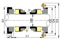
Vulcan manufacture and stock a range of elastomer diaphragm double-ended seals, with boot stationaries at oil side and bezel seats at impeller side, to suit the seal chamber of various Tsurumi\* submersible pumps. Type 260B seals are supplied complete with bezel plates for the inboard seat.
