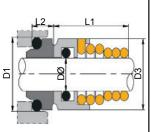
Vulcan manufacture and stock 38mm 'O'-Ring mounted conical spring seals, in clockwise and anti-clockwise rotation, to suit the housing dimensions of common Sterling Sihi® pumps.
