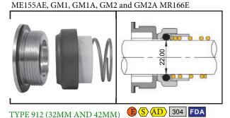
Type 912-32mm and 42mm multi-spring seal kits, designed to suit LKHI, LKHP, LKHSP and LKH 100 series multi-stage series pumps. Please contact us for wear-ring and lip seals sets for these pumps.
