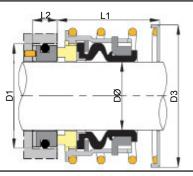
Vulcan manufacture a wide range of differing elastomer diaphragm seals with 'O'-Ring or boot mounted stationaries, to suit the specific dimensions required by various Idex\* Viking\* pumps, of which the Vulcan Type V4 1.1/4" shaft size is a common example. Please contact us with O.E.M. details for cross reference and identification, for any other seal assembly required for this popular brand of pumps.
