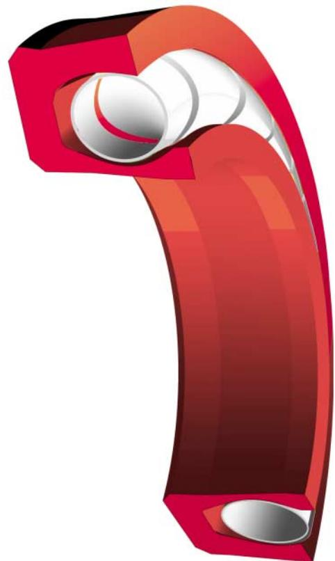
*Reversing pressures require a double cavity piston with back-to-back seals.*
