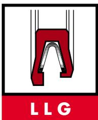
These are used as standard face seals with higher temperature capabilities than elastomeric seals and lower seating load requirements than metal seals. These high conformity seals are an excellent option when flange separation and/or non-parallelism is a concern.
