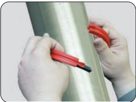
1. Open the seal, install it around the shaft
