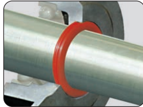
3. Replace the old seal, making sure the split joint faces upward
