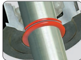
4. Replace the old seal, making sure the split joint faces upward
